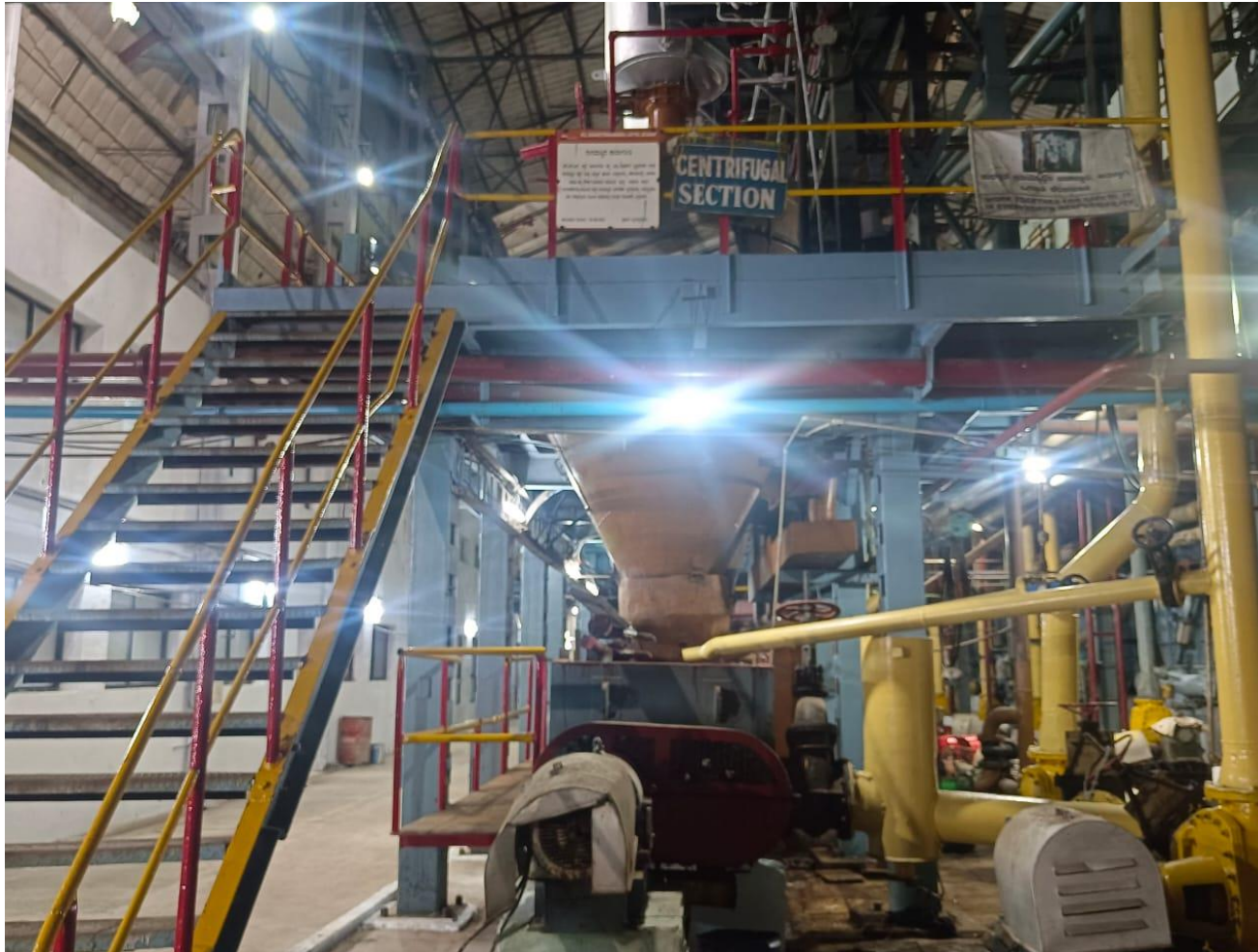
Picture 2: (a) Centrifugal section used for separation of sugar crystals from the molasses (b) Pan boiling section: sugar is extracted from mother liquor through crystallization
