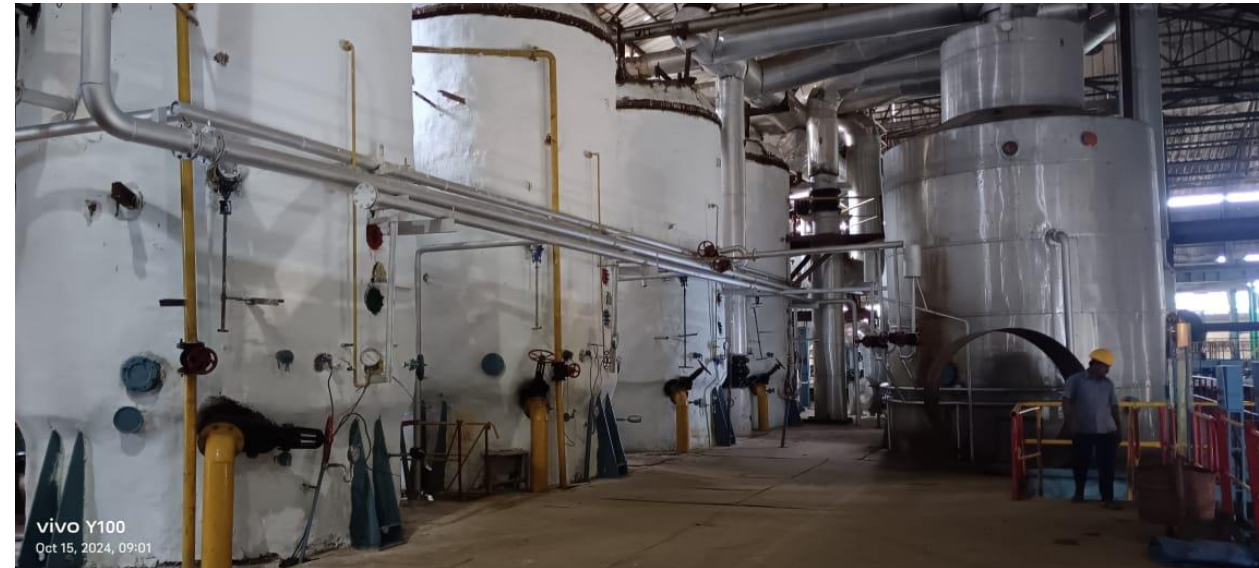
Picture 3: (a) Mill house where the cane is crushed to extract juice and (b) Evaporator section: responsible for converting diluted sugar juice into raw sugar and molasses
